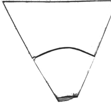
Figure 4. The crack path in the Plexiglas wedge under tension loading.
