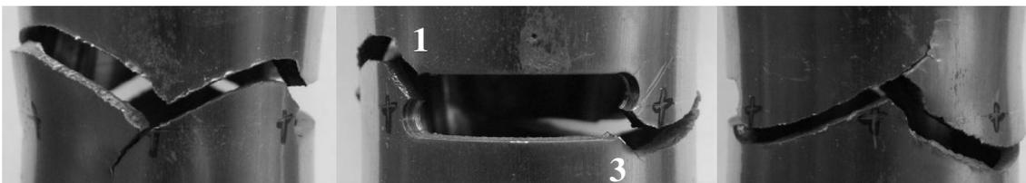
Figure 12. Crack path under out-of-phase loading with a phase angle of  $90^\circ$  with  $(N; M_T)=(18 \text{ kN}; 272 \text{ Nm})$
