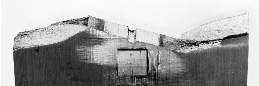
Figure 5. Fracture surface of a 19 mm thick DTD 5050 aluminium alloy mixed Modes I and II fracture toughness test specimen.
