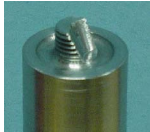
Figure 3. Flute tool geometry used to make the FS welds.
