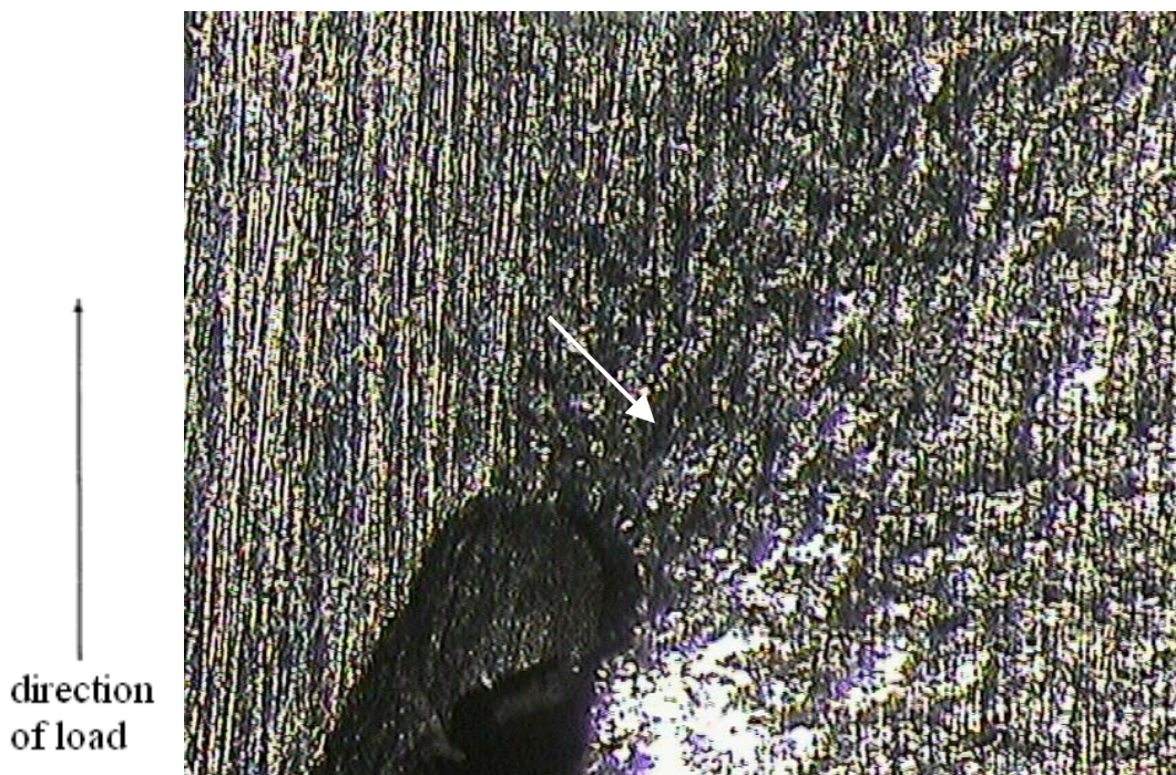
Figure 2. Crack path under mixed mode I+II in FeP04 steel for P_a = 8 kN and \varphi = 60^\circ
