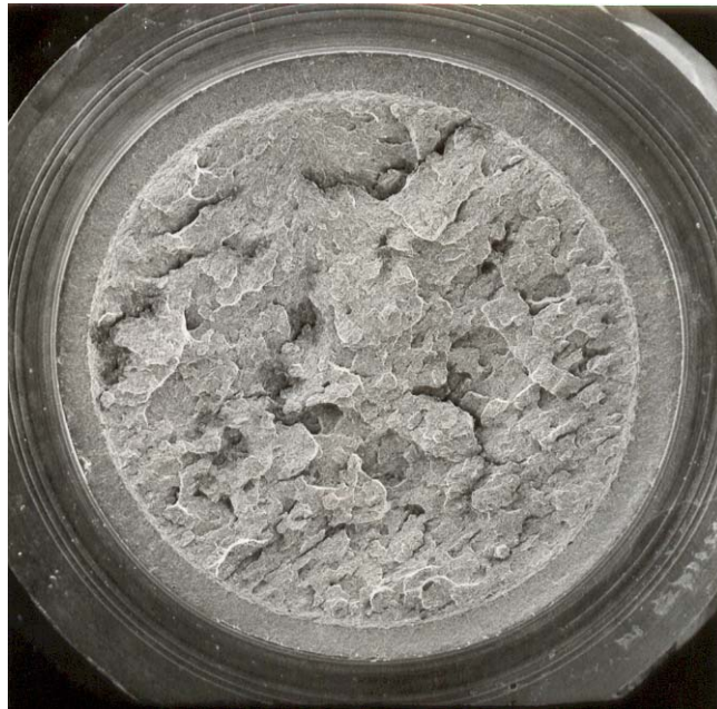
Figure 1. Fractured surface of cylindrical tensile test specimen with precracked circumferential V notch, SEM micrograph, magnification 10 x
