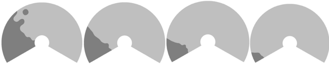
Figure 2 Breathing behaviour of fully loaded cracked shaft: load rotated by 60°, 90°, 120° and 150°. In dark zones contact between crack faces occurs.
