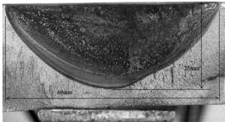
Fig. 3b: Crack path of crack no. 2 in Fig 3a
