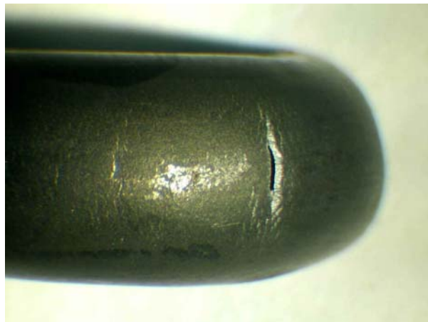
Figure 7. Transversal cracks initiated inside the welded area, within the tube bend.
