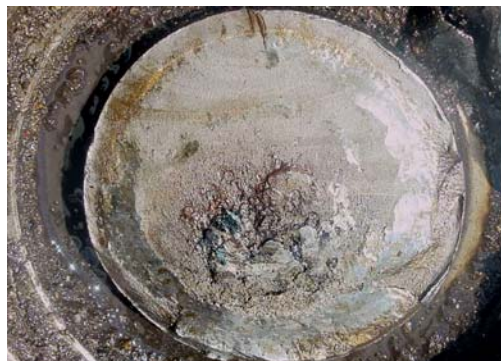
Figure 1. Broken tank wagon axle from a severe derailment, Romania, 15.08.2004 [1].
