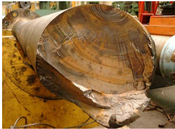
Figure 1 - Fatigue fracture surface and final fracture.
