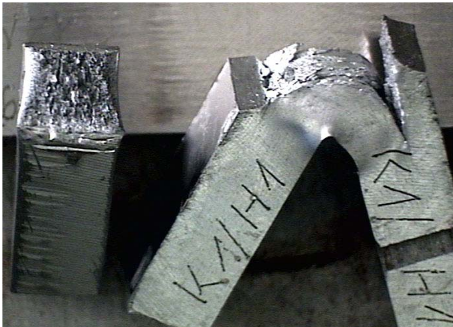
Figure 2. Typical Charpy tests fracture surfaces of the top (on the left) and the bottom (on the right) parts of exploited pipe
