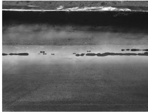
Figure 4. Cracks initiated along the inner corner of the tube. Dark regions are cracks highlighted using a dye-penetrant solution.
