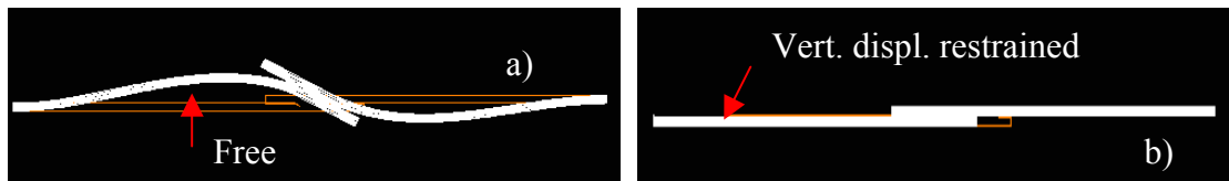
Figure 6. Deformed numerical models without (a) and with (b) antibending system.
