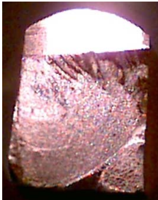
Figure 4. Surface of fatigue fracture of the specimen under bending with torsion in AlCuMg1 alloy for R = -0.5 , \alpha = 45^\circ and N_f = 3.5 \cdot 10^4 cycles
