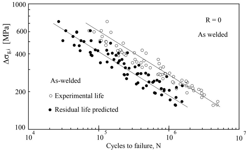
Figure 4: Fatigue strength data and residual life estimates. Residual life determined by assuming the initial crack length  $a_i = 0.3\text{mm}$  and the crack propagation along the direction ( $\theta = 22.5^\circ$ ).  $Y=1.122\sqrt{\text{sec}(\pi a/t)}$ ; coefficients in the Paris law:  $m=3.0$ ;  $C=0.183 \times 10^{-12}$ , (N and mm as units), (Gurney, 1991).
