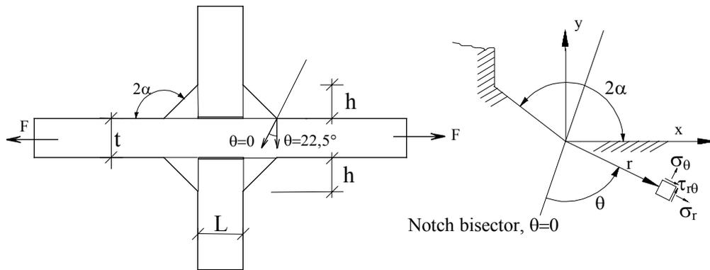
Figure 1. Typical welded joint geometry and local coordinate system.
