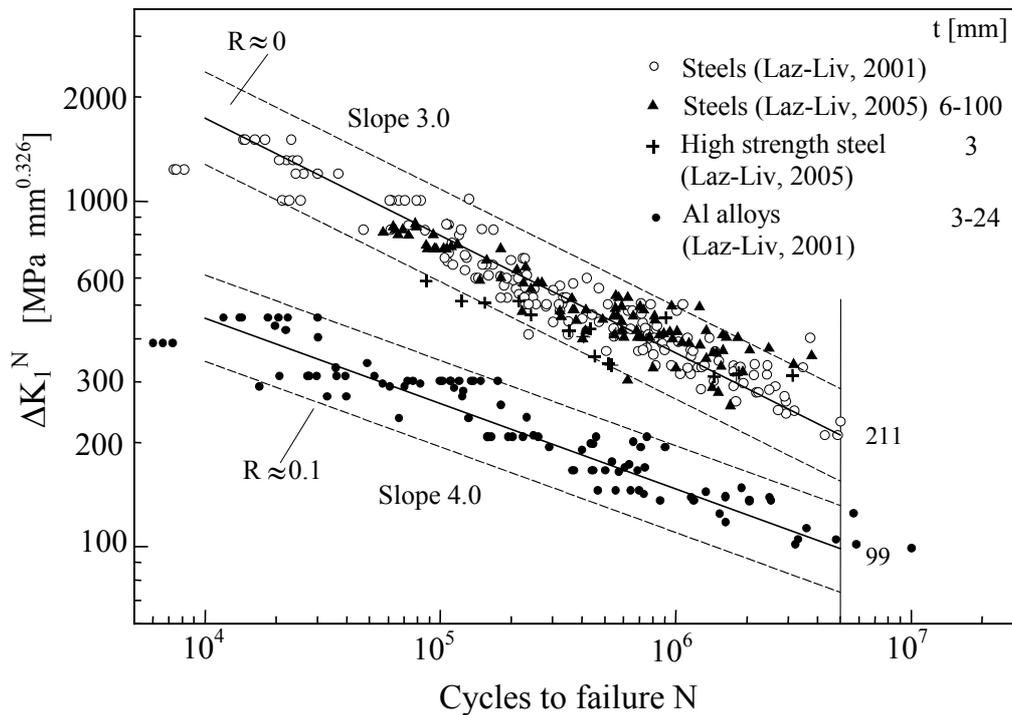
Figure 3. Fatigue strength of welded joints made of steel and aluminium as a function of mode I notch stress intensity factor. Scatter bands defined by mean values plus/minus 2 standard deviations. All failures from the weld toe, in the presence of  $2\alpha=135$  degrees.
