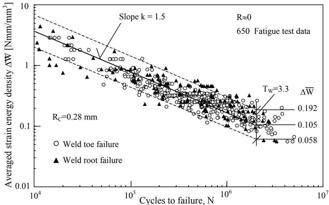
Figure 6: Fatigue strength of fillet welded joints as a function of the averaged local strain energy density; scatter band defined by mean value  $\pm 2$  standard deviations; main plate thickness ranging from 6 to 100 mm; crack initiation at weld toe or weld root.
