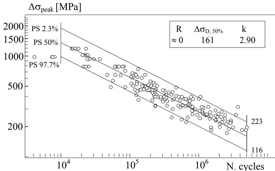
Figure 6: fatigue strength of fillet welded joints in structural steel in terms of elastic peak stress evaluated at the weld toe.
