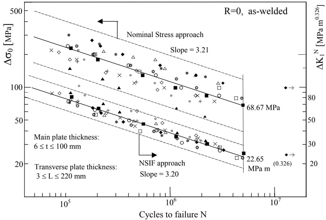
Figure 2. Fatigue strength data in terms of nominal stress range or the mode I NSIF range (from Lazzarin and Tovo, 1998. Original series from Maddox, 1987, and Gurney, 1991). All joints re-analysed here were as-welded, with a V-notch angle at the weld toe equal to 135 degrees. Scatter bands defined by mean values plus/minus 2 standard deviations.
