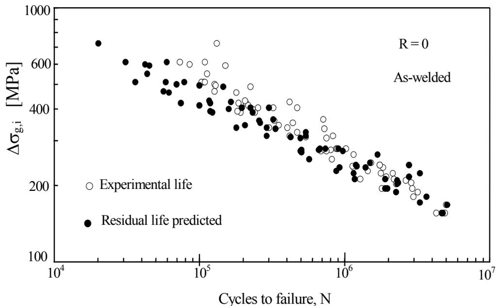
Figure 5: Fatigue strength data and residual life estimates. Residual life determined by assuming the initial crack length  $a_0 = 0.3\text{mm}$  and the crack propagation along the direction  $\theta = 22.5^\circ$ .  $Y=1.122\sqrt{\text{sec}(\pi a/t)}$ . Coefficients in the Paris law:  $m=4.0$ ;  $C=0.2046 \times 10^{-15}$  (N and mm as units), (Gurney 1991).
