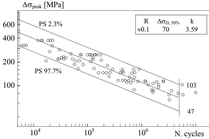
Figure 7: fatigue strength of fillet welded joints in aluminium alloys in terms of elastic peak stress evaluated at the weld toe.
