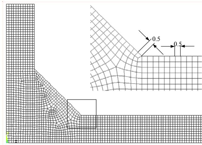
Figure 5: adopted mesh pattern for the stress analysis of cruciform joints. (Main plate thickness  $t=12$  mm, adopted element size: 0.5 mm)
