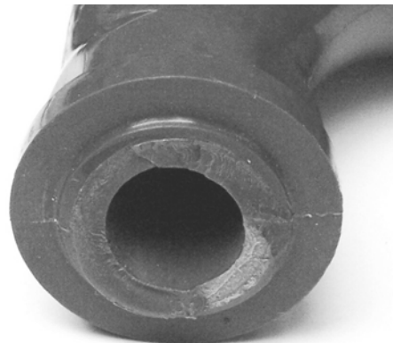
Figure 8. Crack surface of plastic domestic tap.
