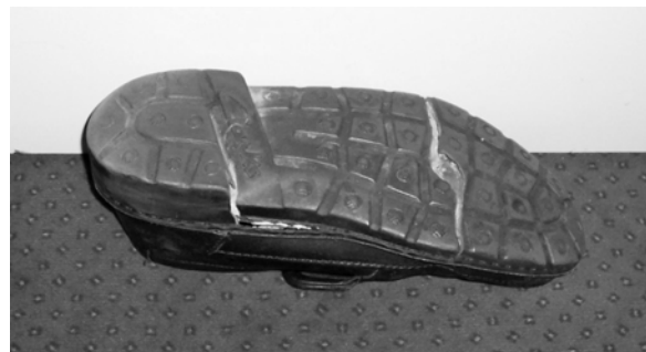
Figure 18. Cracks in sole of walking shoe.
