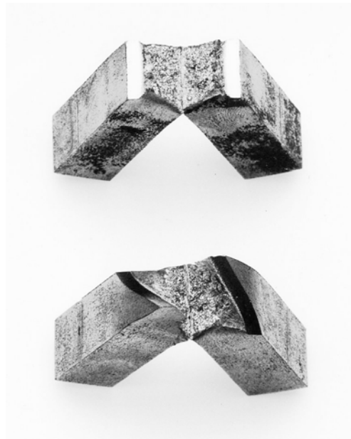
Figure 12. Fracture appearance of mild steel Charpy specimens tested at 10° C. Top, standard specimen, \beta = 90^\circ . Bottom, angle notch specimen, \beta = 45^\circ .
