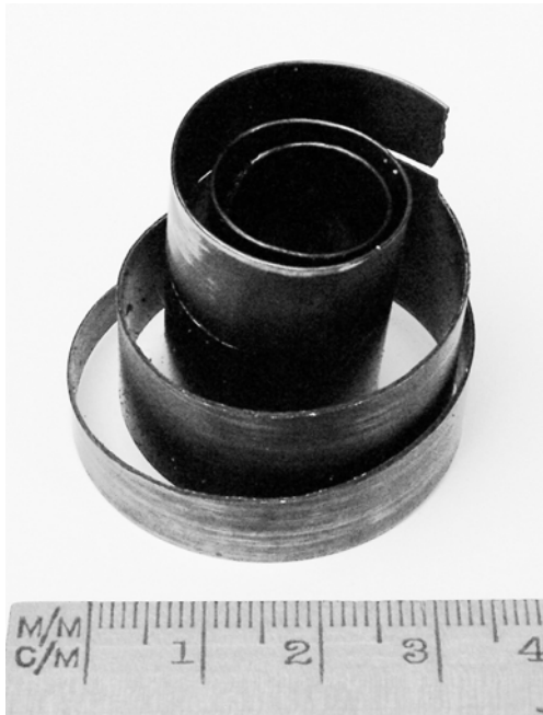
Figure 11. Centre portion of failed wall clock mainspring.
