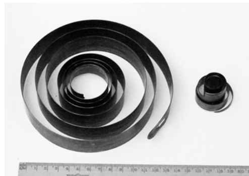
Figure 9. Wall clock by John Davidson, Coatbridge. Figure 10. Failed wall clock mainspring.
