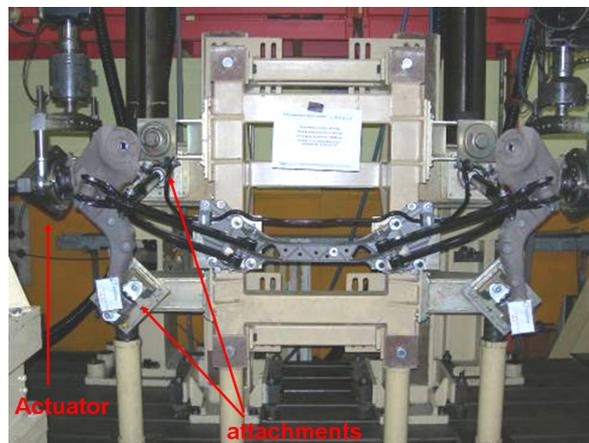
Figure 2: Component test arrangement showing details of fixturing close up.
