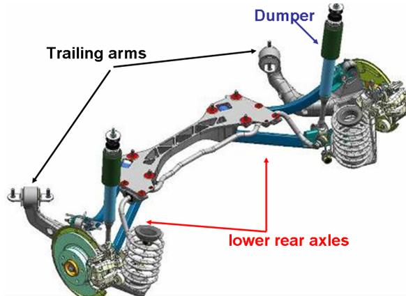
Figure 1: Automotive rear chassis system.
