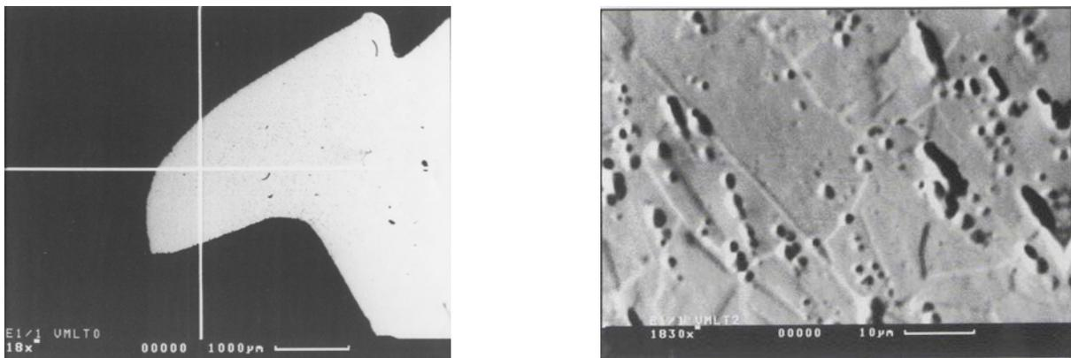
Figure 15: No twins detected below the surface of a stainless steel screw of the triple indicator.
