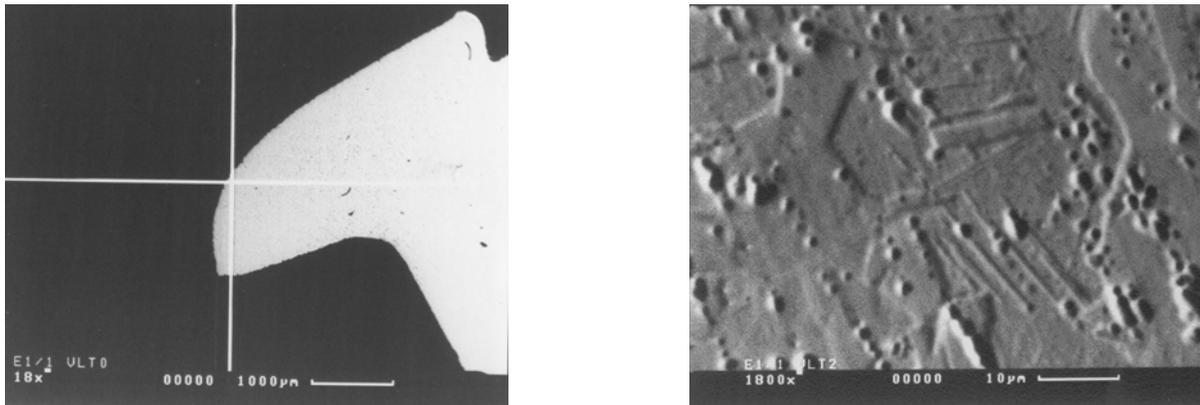
Figure 14: Twins in isolated grains at another point of the surface of a stainless steel screw of the triple indicator.
