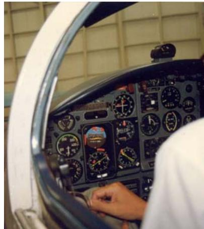
Figure 9: The triple indicator was positioned on the upper left corner of the airplane dashboard.
