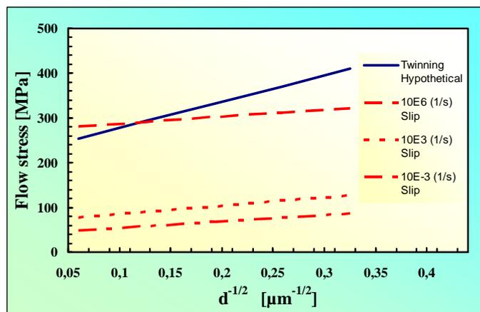
Figure 10: Hall-Petch plots for plastic flow slip ( $10^{-3}$ ,  $10^3$  and  $10^6$  s<sup>-1</sup>) and twinning (Hypothetical) for Cu, as suggested by Meyers *et al.*, [13].
