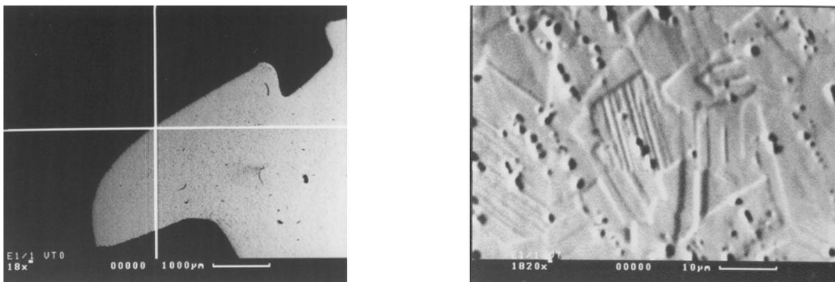
Figure 13: Twins in isolated grains at the surface of a stainless steel screw of the triple indicator.
