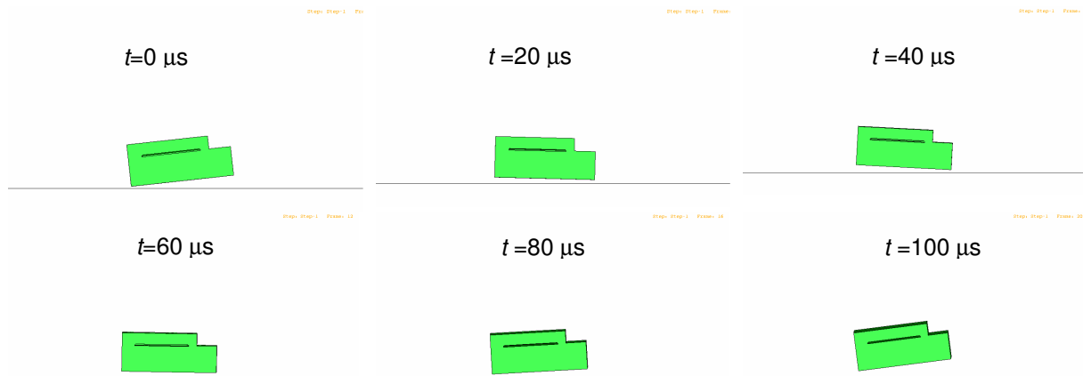
Fig. 2 - Drop height 150 cm; impact angle 10^\circ . Snapshots of the bouncing die, taken every 20 \mu\text{s} after the impact
