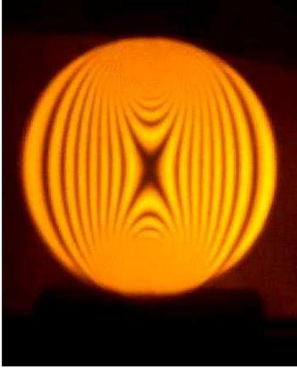
Fig. 5. Isochromatic fringes in calibration disk.
