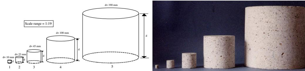
Figure 1. (a) Geometries of the five different concrete specimens; (b) overall view of the five specimen sizes.
