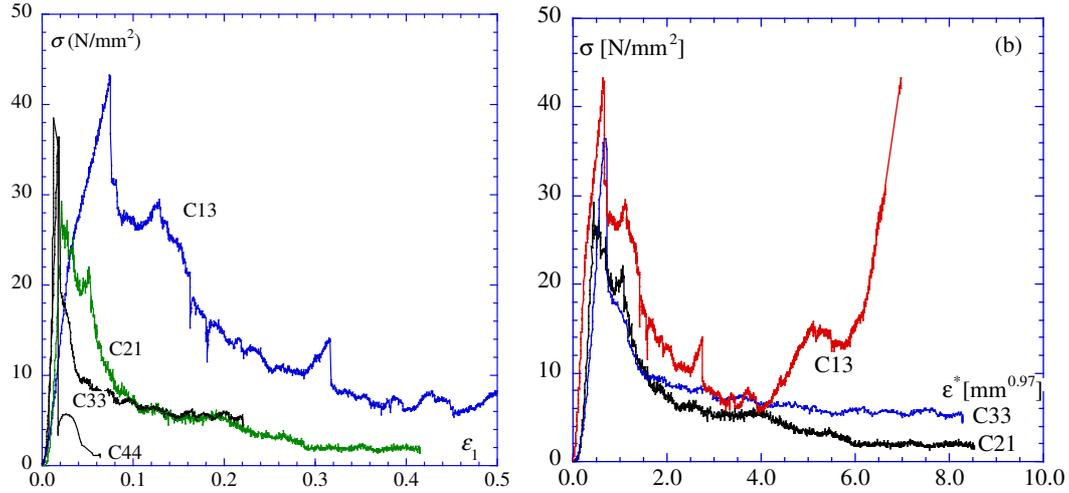
Figure 3. (a) Stress-strain curves for four different cylindrical specimen sizes; (b) Stress vs renormalized strain for four different specimen sizes  $D=2.03$ .
