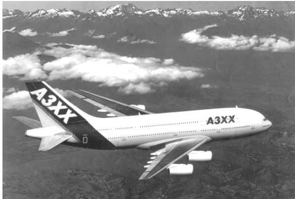
Fig. 1.1 – The Airbus A380 has 400 m 2 of upper fuselage made of GLARE. It will permit to save up to 25% in weight respect to a conventional structure.
