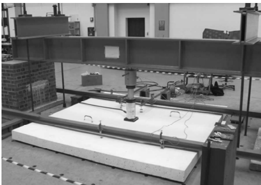
Figure 1: Slab with the load frame and the instrumentation for a single load [5].
