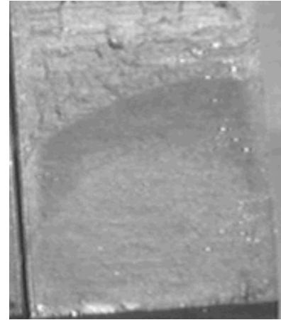
Fig 10. Fracture surface of the case hardened steel tested in the near-threshold region.
