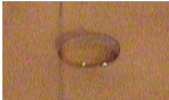
Fig. 4. Photograph of distilled water drop on polyimide film surface P? -1E after 28 month exposure on the orbital space station "Mir".
