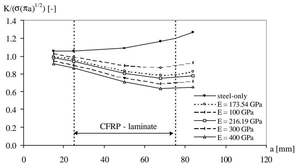
Figure 6. Stress intensity factor vs crack length as function of the patch Young's modulus.
