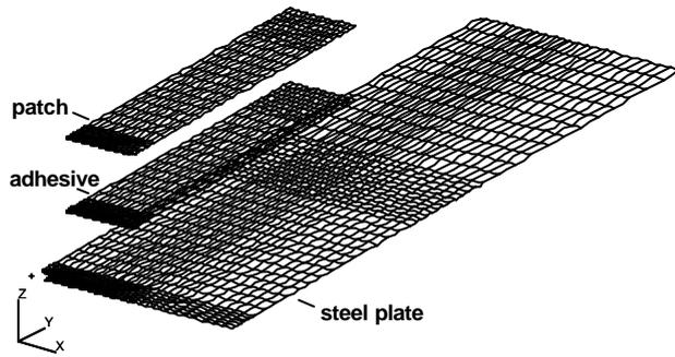
Figure 4. Three layer F.E.M 1/8 model.
