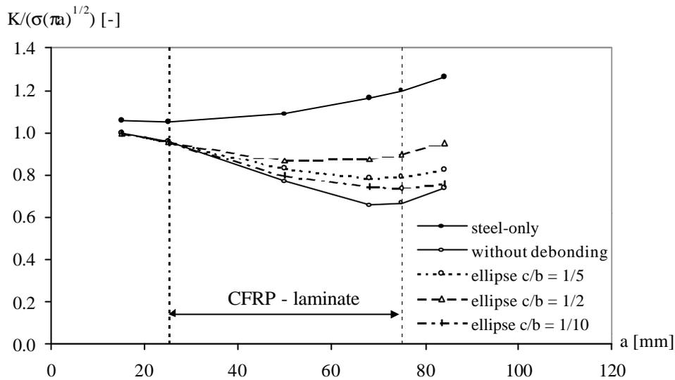
Figure 9. Stress intensity factor vs crack length as function of the patch debonded area.
