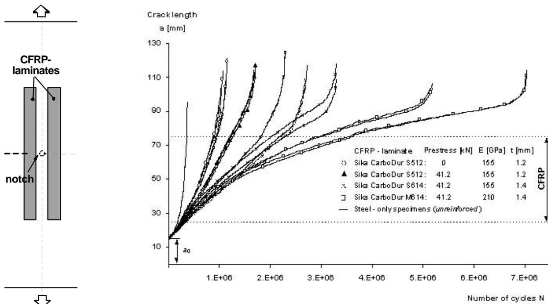
Figure 1. Notched plate. Figure 2. Crack length vs. cycles for the notched plate.
