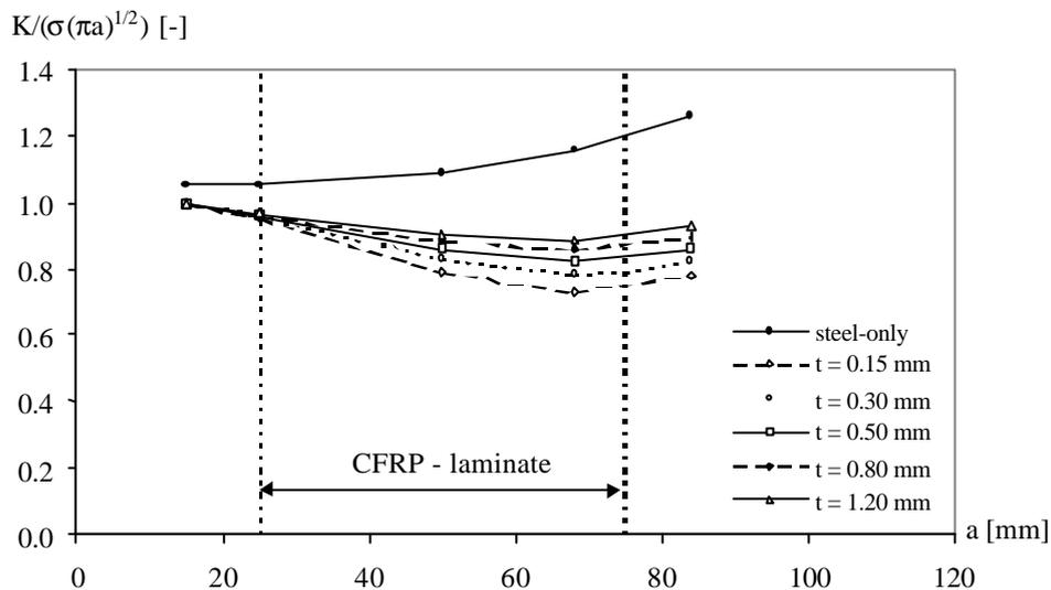
Figure 7. Stress intensity factor vs crack length as function of the adhesive thickness.
