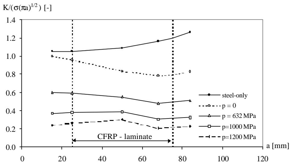
*Figure 8. Stress intensity factor vs crack length as function of the pretension level.*
