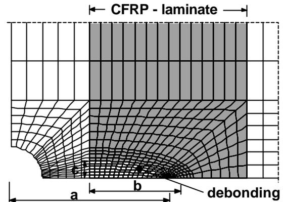
Figure 5. Detail of F.E.M. model.
