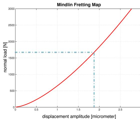
Figure 4: Fretting Map using a COF equal to 0.1.
