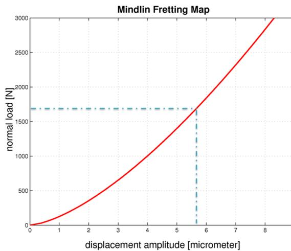
Figure 5: Fretting map using a COF equal to 0.3
