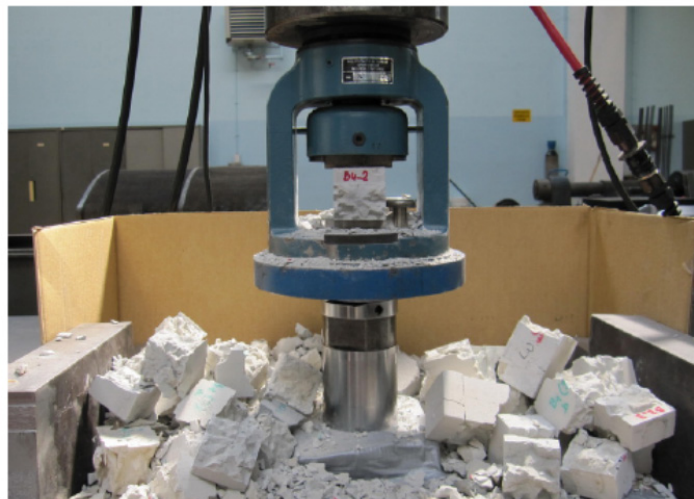
Figure 2: Compression test configuration.
