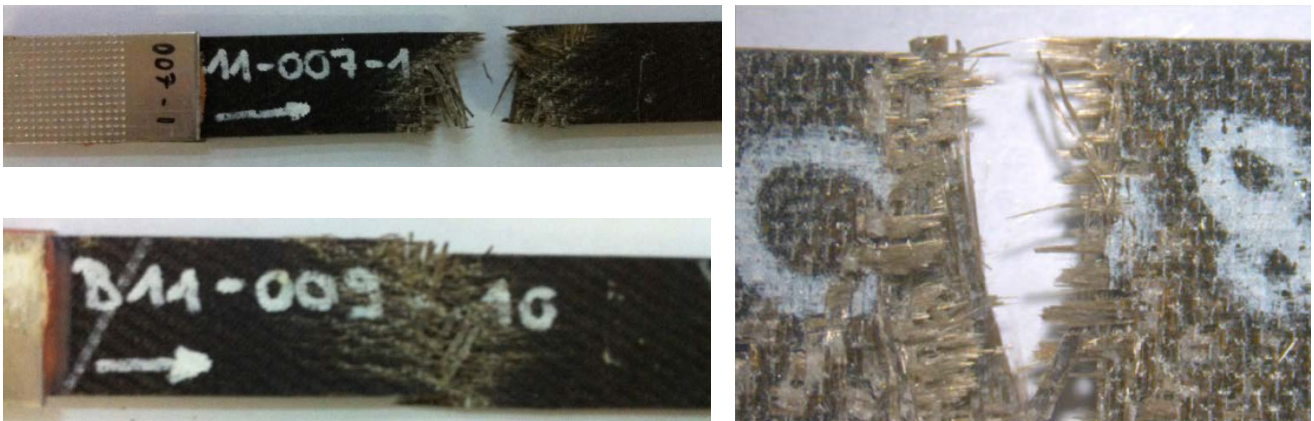
Figure 10: Exemplarily pictures of a fractured specimen with fabric reinforcement of the type twill weave 2/2 in warp direction ( 0^\circ ). Upper and lower left: Picture taken by a normal digital camera. Right: Picture taken under the optical microscope.
