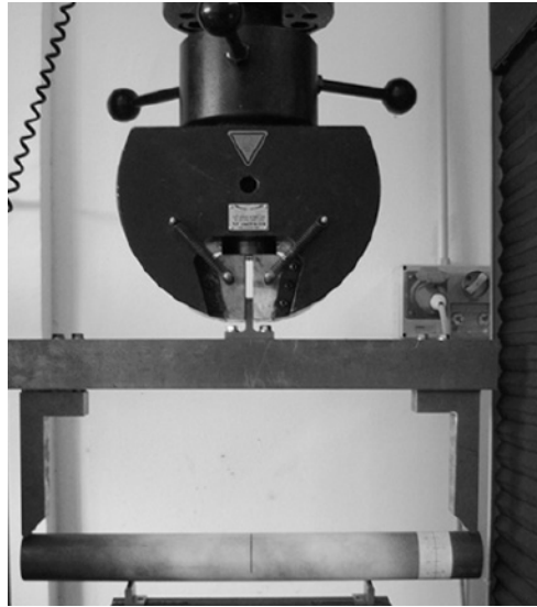
Figure 3: Pipe four point bend loading fixture. Picture shows pipe surface prepared with stochastic pattern for DIC measurement, [4].
