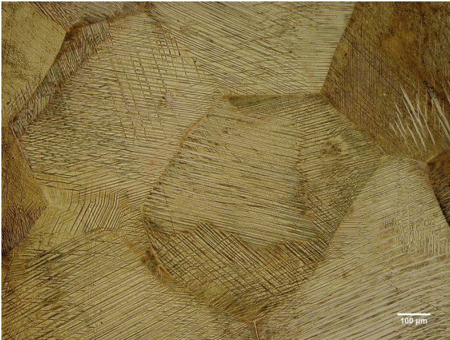
Figure 6a: 100X LOM micrograph of a sample deformed up to 7.5%: strips of variously oriented martensite.
