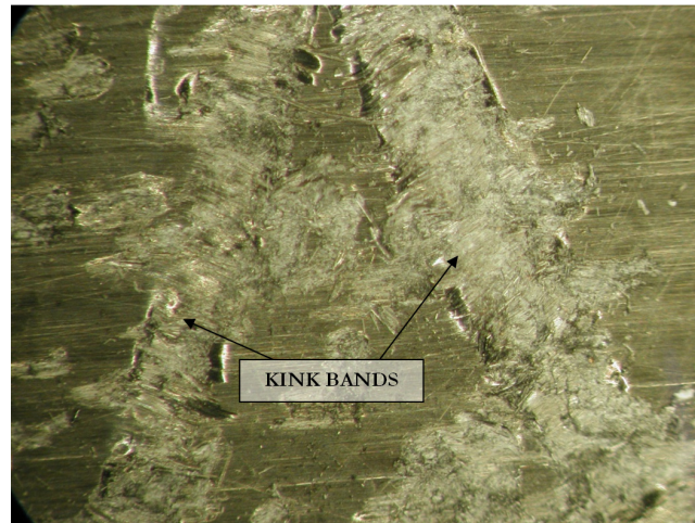
Figure 6: Microscope photograph (detail) of E13 sample gage section (front view).
