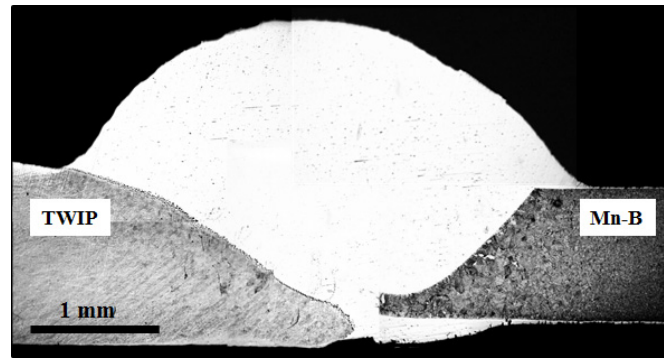
Figure 1: Overview of a butt welded joints between TWIP and Mn-B steels.
