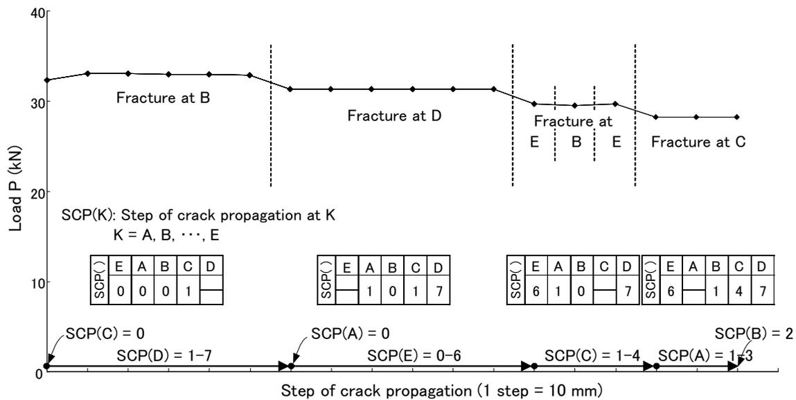
Figure 4. Numerical results on multistage strength degradation due to crack propagation and change of failure mode in a notched beam
