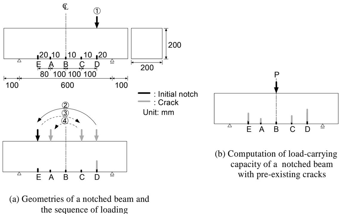
Figure 2. Scheme of numerical studies on a notched beam
