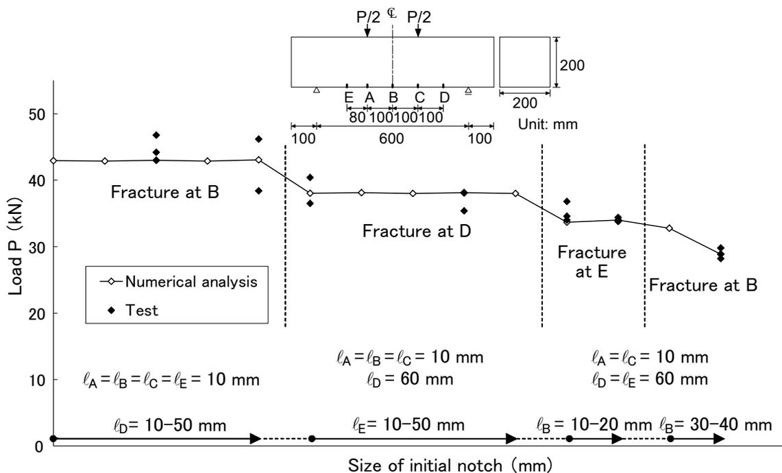
Figure 1. Numerical and experimental results on multistage strength degradation due to change of failure mode in bending tests of notched concrete beams [4]
