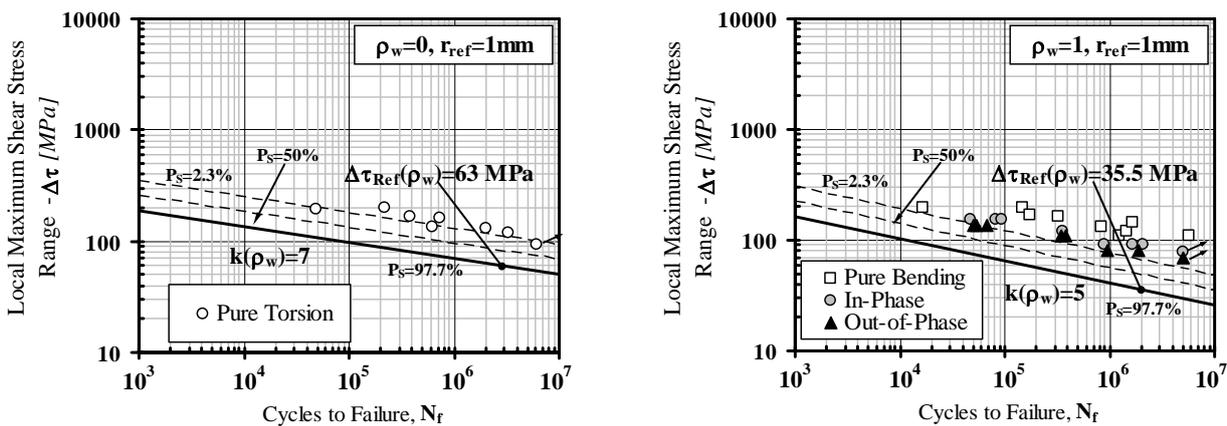
Figure 5. Comparison between the design curves supplied by the MWCM, applied along with the reference radius concept, and the considered experimental results generated by testing “thin and flexible” as-welded samples made of aluminium.
