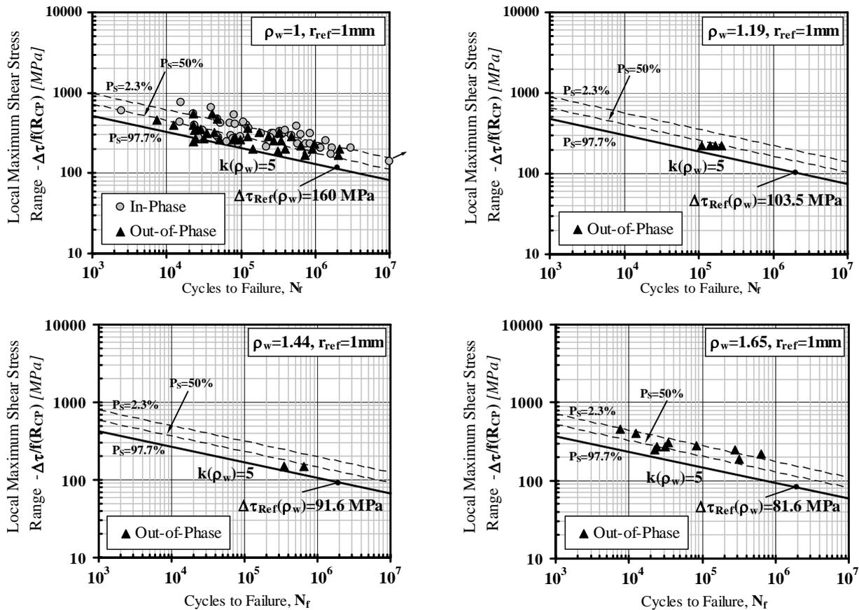
Figure 4. Comparison between the design curves supplied by the MWCM, applied along with the reference radius concept, and the considered experimental results generated by testing “thin and flexible” samples made of steel.
