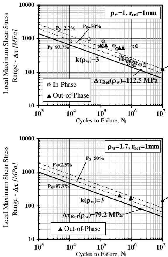
Figure 3. Comparison between the design curves supplied by the MWCM applied along with the reference radius concept and the considered experimental results generated by testing “thick and stiff” as-welded samples made of steel.
