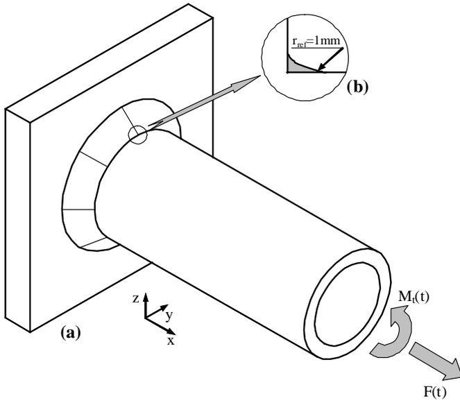
Figure 1. Tube-to-plate welded joint subjected to combined tension/torsion.
