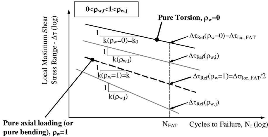
Figure 2. Modified Wöhler Curve Diagram.
