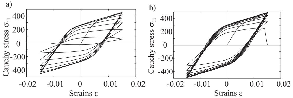
Figure 1: Uniaxial tension test: Stress-strain response as predicted by the novel brittle damage law (3D-computation), a)  $(H_\Gamma, B_\Gamma) = (250.0, 10.0)$ , b)  $(H_\Gamma, B_\Gamma) = (1250.0, 50.0)$ .
