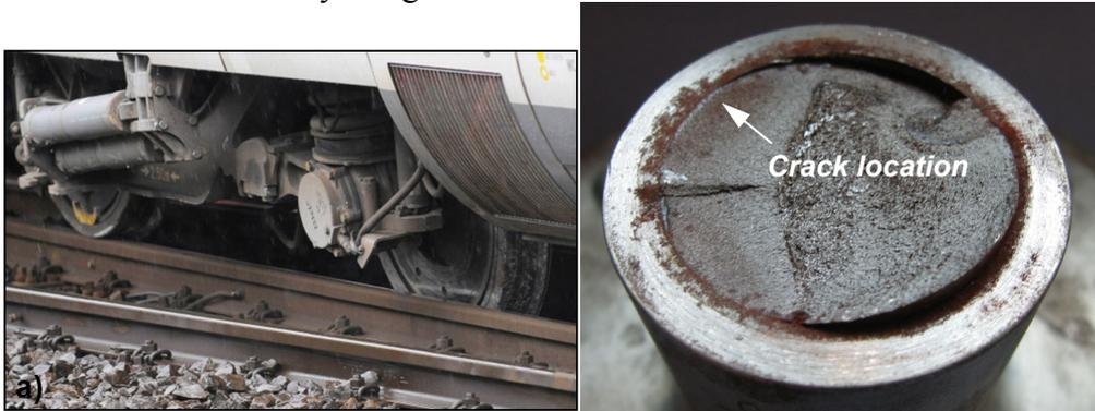
Figure 1. Shaft failure of ICE3 train caused by fatigue crack [1] (left); fatigue fracture surface of shrink-fitted assembly subjected to rotating bending [2] (right).
