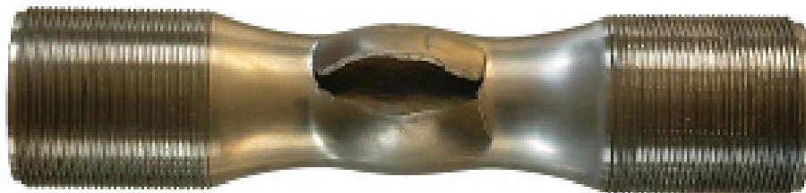
Figure 4: Specimen broken in tension-internal pressure equibiaxial regime (CEAT, TA6V)
