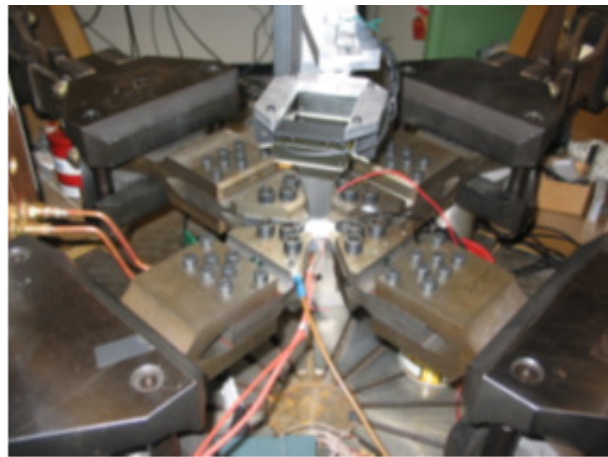
Figure 5b: Specimen mounted on the biaxial device
