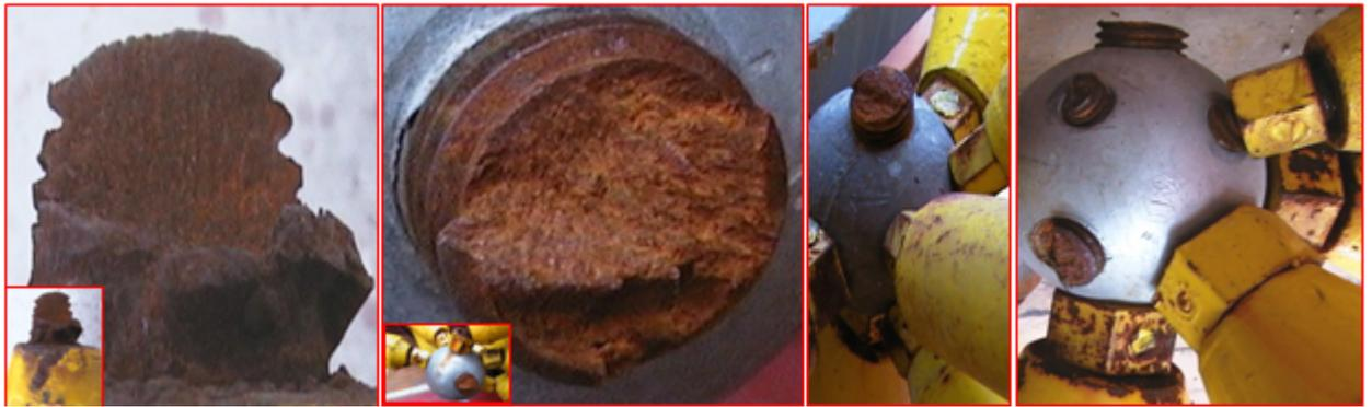
Fig. 5 Shear fracture (corrosion)
