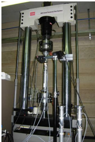
Figure 5 – Experimental set-up of the torsional tests
