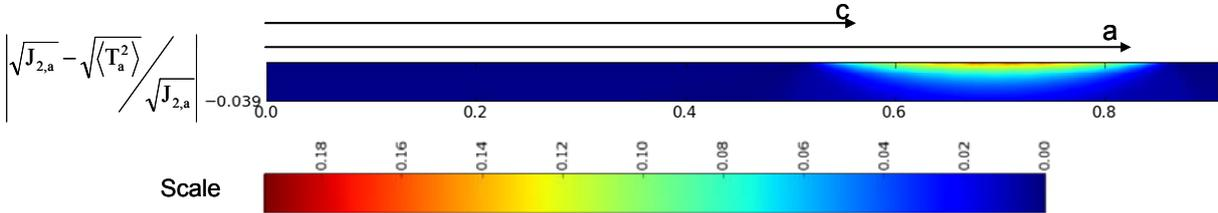
Figure 4: Estimation of the proportionality of the stress field induced by a cylinder plane contact under varying tangential load.
