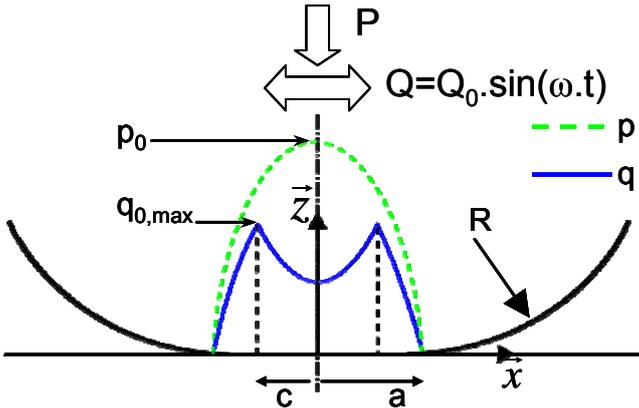
Figure 1: Surface traction distribution  $p$  and  $q$  for  $Q(t)=Q_0$  in a cylinder plane contact and definition of the maximal pressure  $p_0$ , the maximal surface shear traction  $q_{0,max}$ , the semi contact width  $a$  and the semi sticking zone width  $c$ .
