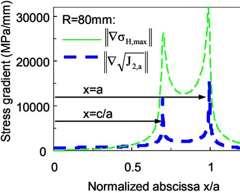
Figure 2: Comparison of the gradients of  $\sigma_{H,max}$  and  $\sqrt{J_{2,a}}$  for a cylinder plane contact using two cylinder radii.
