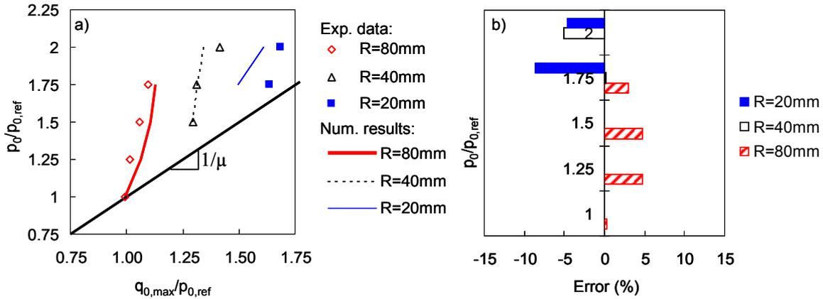
Figure 7: Variable process volume approach [8],  $h=6.2$  a) Comparison between experimental and numerical initiation boundaries in a  $p_0$ - $q_{0,\text{max}}$  diagram. b) Error between experimental and numerical results.
