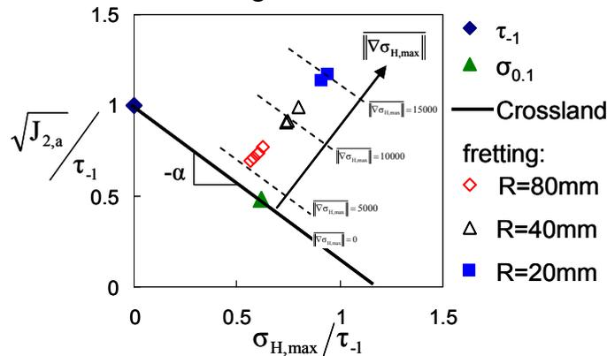
Figure 6: Experimental results plotted in a  $\sqrt{J_{2,a}} - \sigma_{H,max}$  diagram compared to the fatigue strength computed using to the Crossland criterion.
