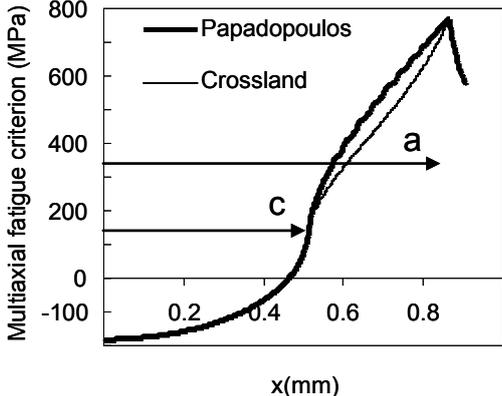
Figure 3: Comparison of the Crossland and the Papadopoulos distribution at the surface of the plane.
