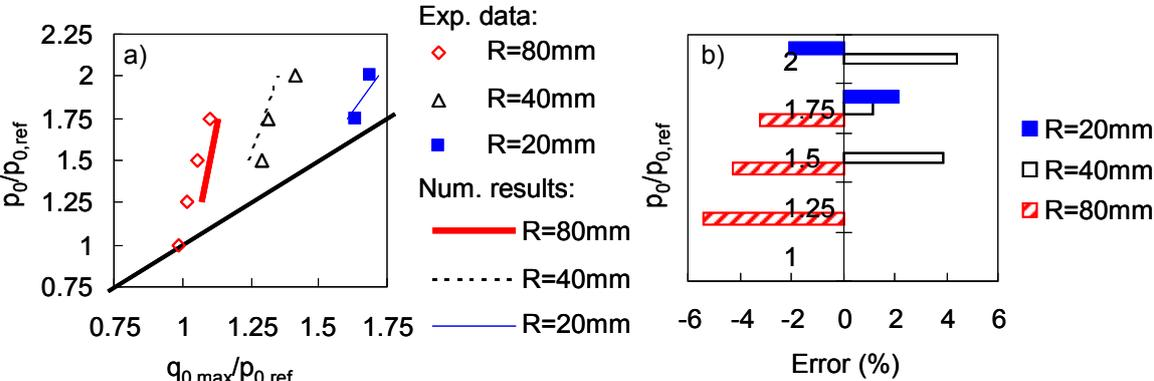
Figure 9: Proposal a) Comparison between experimental and numerical initiation boundaries in a  $p_0$ - $q_{0,max}$  diagram. b) Error between experimental and numerical results.
