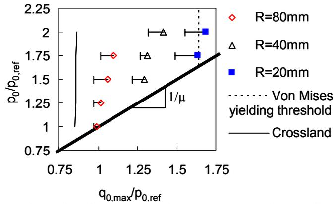
Figure 5: Experimental results showing crack initiation conditions for fretting tests under partial slip regime on Inconel 718 at  $10^5$  cycles. Three crack initiation boundaries are clearly identified for each contact configurations tested. The experimental results are compared to the computations done using the local Crossland multiaxial fatigue criterion.
