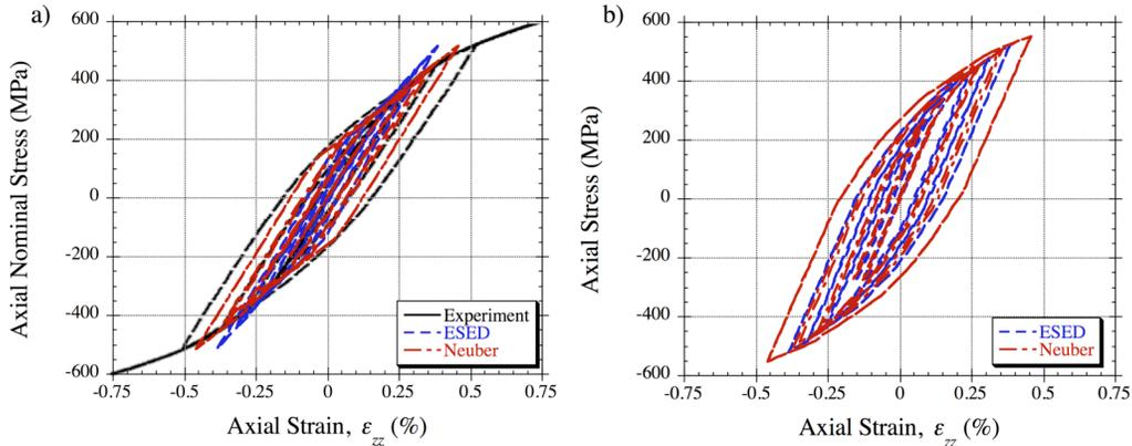
**Figure 2: Incremental step test for (a) the nominal stress versus local strain and (b) the local stress versus strain for the experiment [9], ESED and Neuber models**
