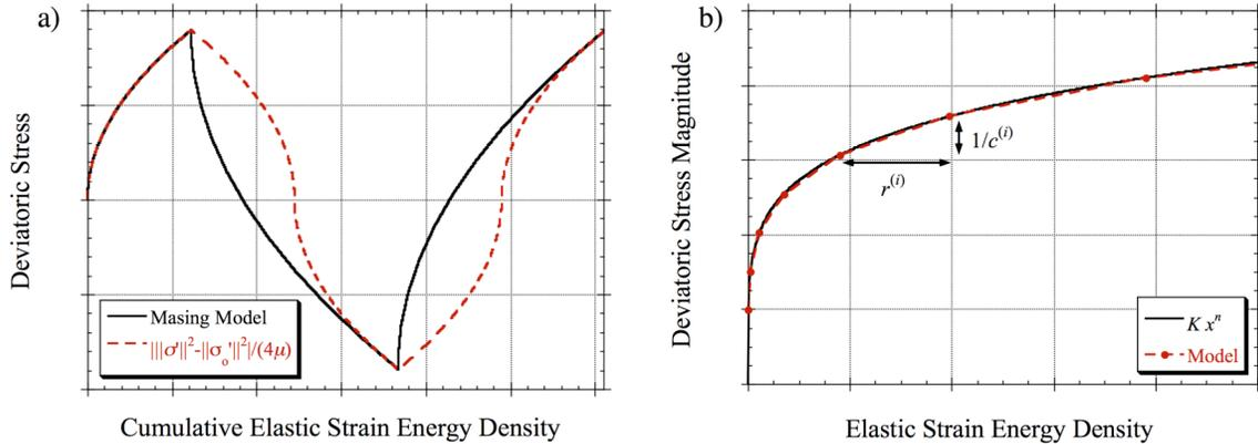
**Figure 1: Deviatoric stress magnitude versus (a) cumulative strain energy density for the Masing and monotonic models for fully-reversed cyclic loading and (b) the elastic strain energy density, illustrating the linearly segmented material model**
