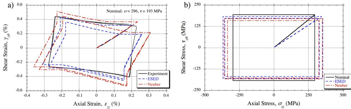
**Figure 3: Multiaxial ‘Box’ loading path illustrating (a) shear strain versus axial strain and (b) the shear stress versus axial stress for the experiment [9], ESED and Neuber models**
