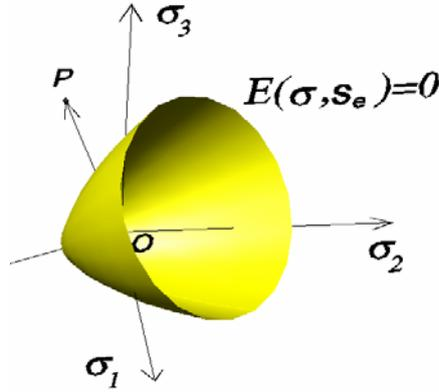
Fig. 1. A schematic view of the endurance function in the principal stress space
