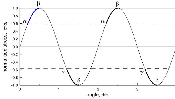
Fig. 3. Constant amplitude cycling loading: zones of damage development
