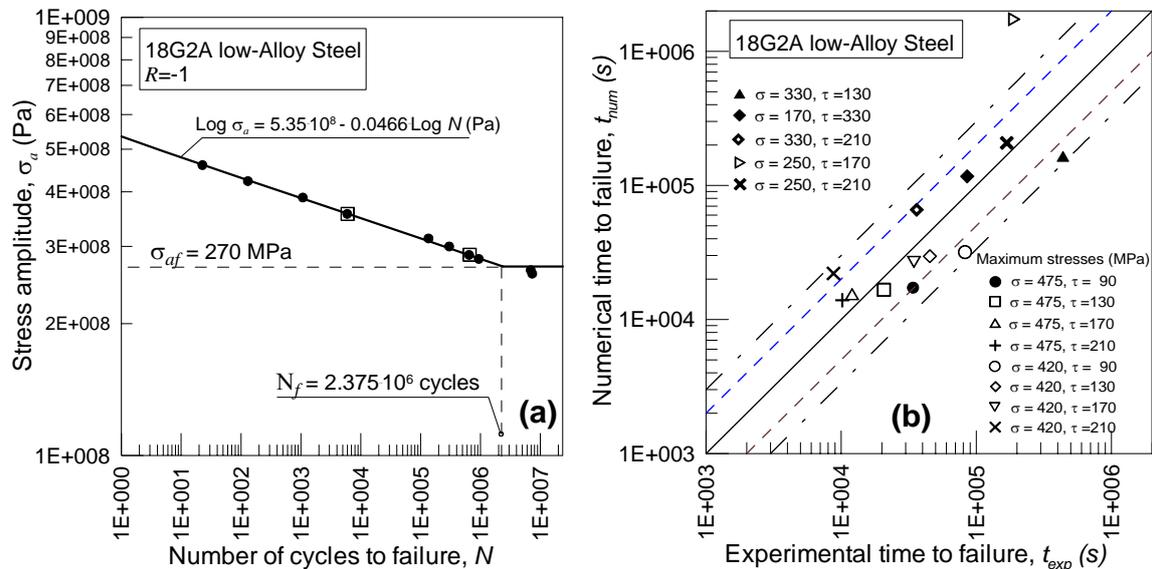
Fig. 4. (a) The Wöhler curve for steel 18G2A: estimation through the present model (dots). The squares indicates the points used for the model calibration. (b) Multiaxial random loading simulation: comparison between experimental [14] and numerical simulations.
