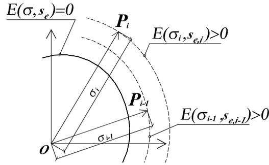
Fig.2. Definition of the endurance function evaluation  $E(\sigma_e, s)$  for the stress states  $\sigma_i$  and  $\sigma_{i-1}$
