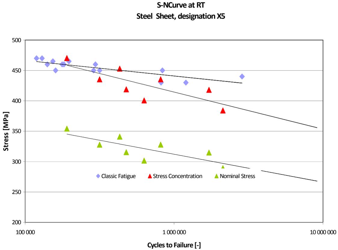
**Figure 6. An Example of S-N Curve of the X5 Steel**
