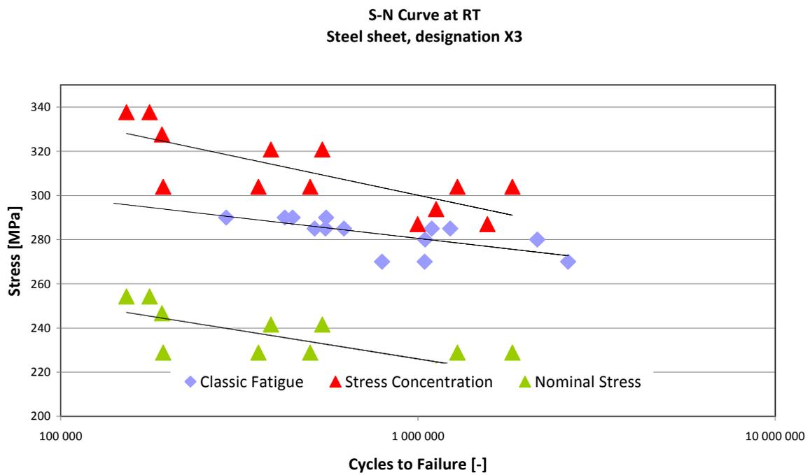
Figure 5. An Example of S-N Curve of the X3 Steel
