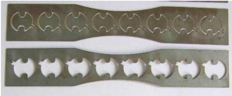
**Figure 2. Miniature fatigue test specimens**
