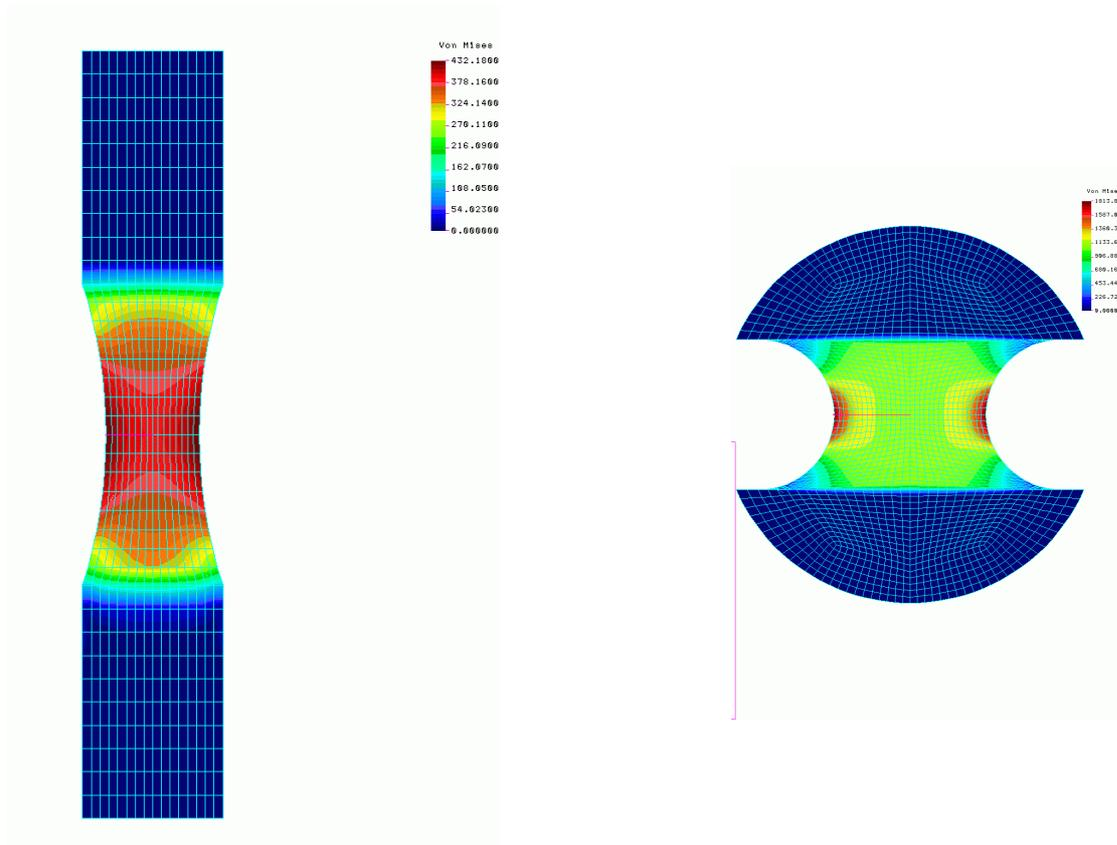
Figure 4. FEM models of classic and miniature test specimens
