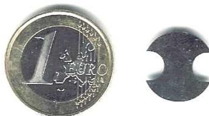
**Miniature Test Specimen for Fatigue Test**
