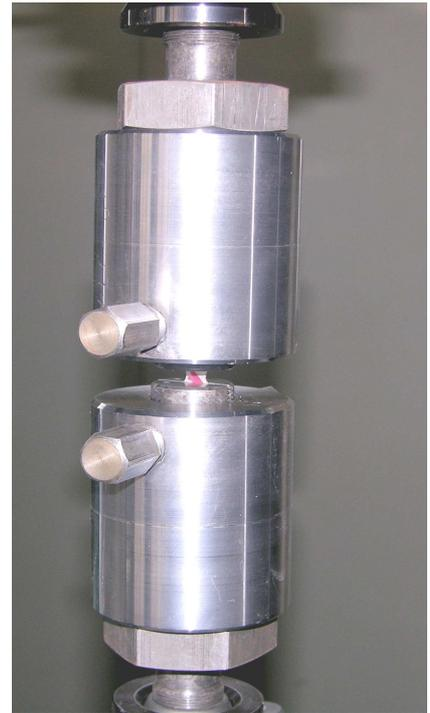
**Figure 3. Miniature test specimens grips**
