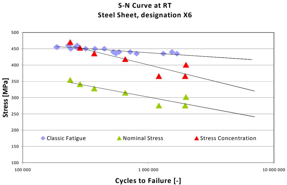
**Figure 7. An Example of S-N Curve of the X6 Steel**
