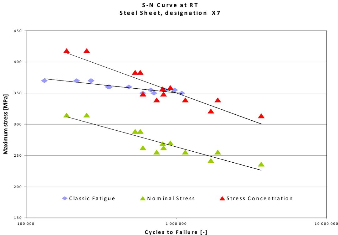
**Figure 8. An Example of S-N Curve of the X7 Steel**
