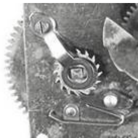
Figure 2. Click work in a mainspring powered clock.
