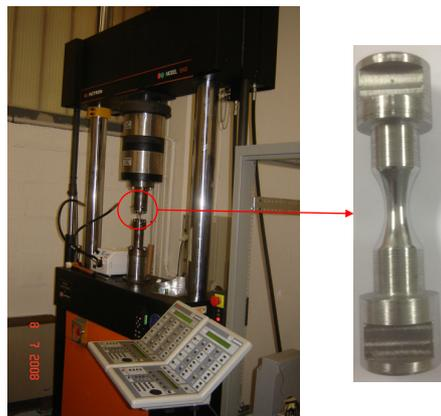
Figure 2 – Experimental tension-torsion device and cylindrical 1045 steel specimen
