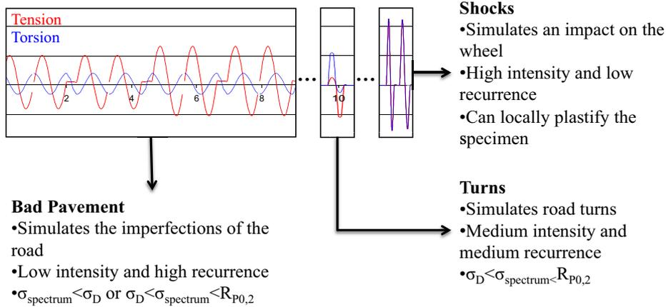
Figure 3 – Sample of loading spectrum used in tests
