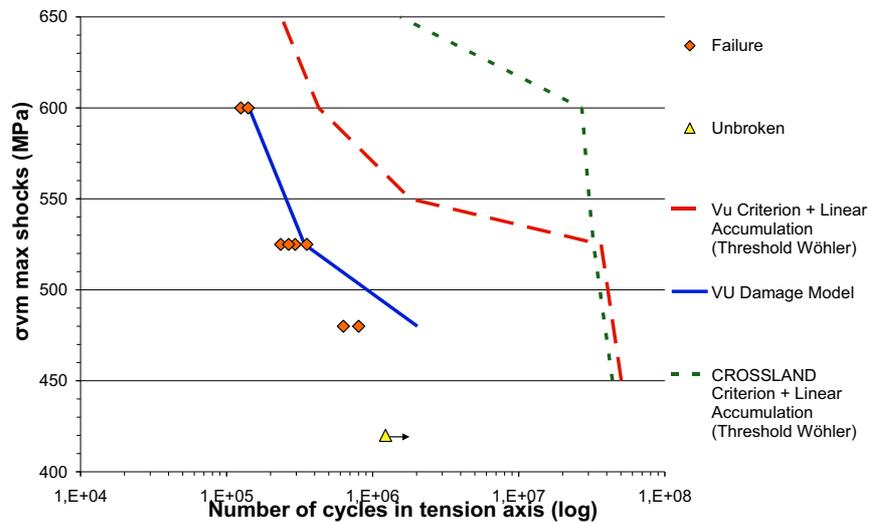
Figure 5 - Comparison of experimental data (1045 steel cylindrical specimens), CROSSLAND Criterion, VU Criterion and VU Damage Model
