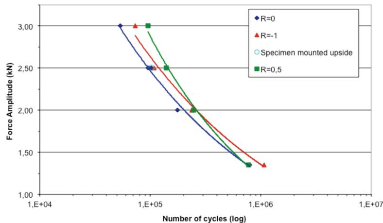
Figure 10 – MS4 tension fatigue tests. Sinusoidal loads with three load ratios  $R=0$ ,  $R=-1$  and  $R=0.5$ . Tests stopped at crack initiation.
