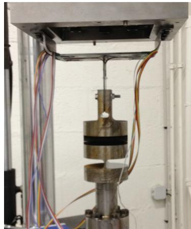
Figure 8 – Experimental devices to MS4: a) Bending, b) Tension (Instrumented)
