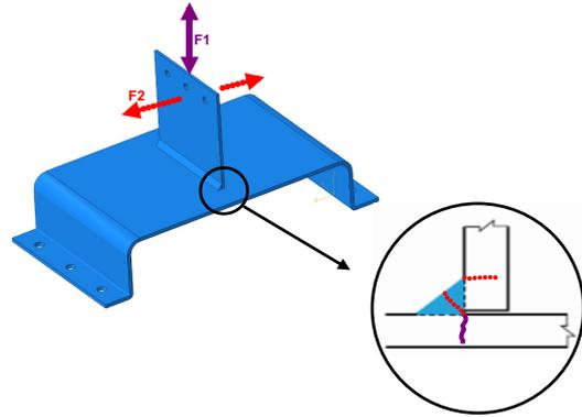
Figure 7 - MS4 study load cases and expected crack location
