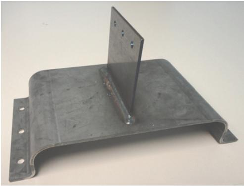
Figure 6 – Welded Specimen “Mini-Structure 4 (MS4)”
