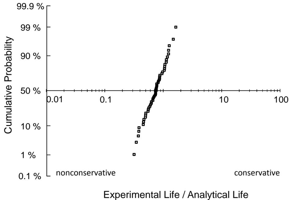
Figure 5. Cumulative probability distribution for tubular specimens.
