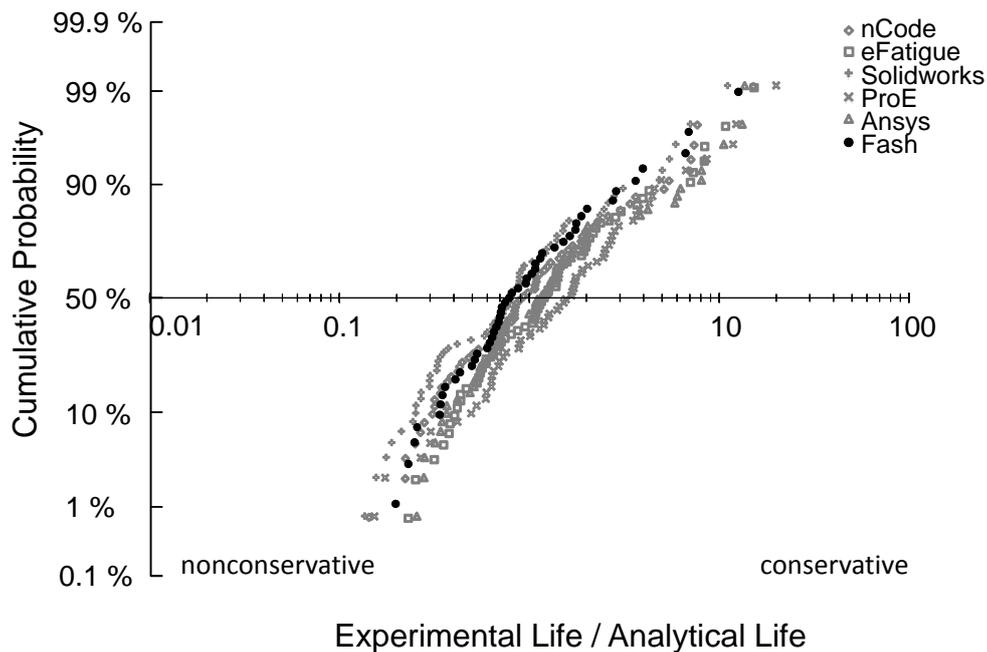
Figure 4. Cumulative probability distribution for in-phase loading.
