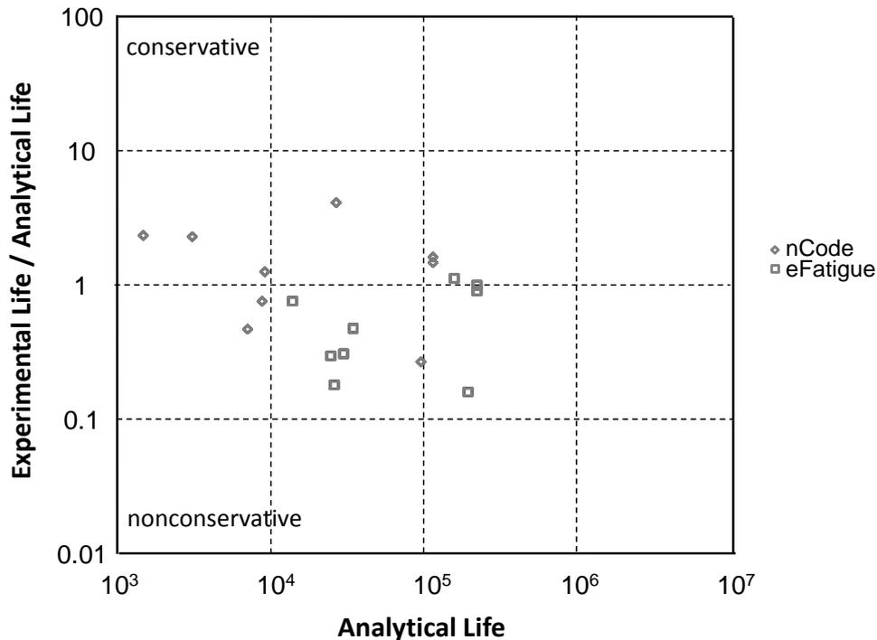
Figure 3. Analytical results for 90 deg out-of-phase loading.
