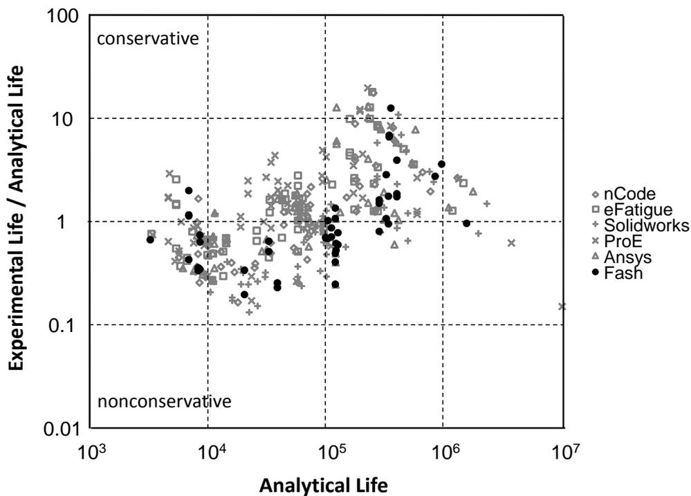
Figure 2. Analytical results for in-phase loading.
