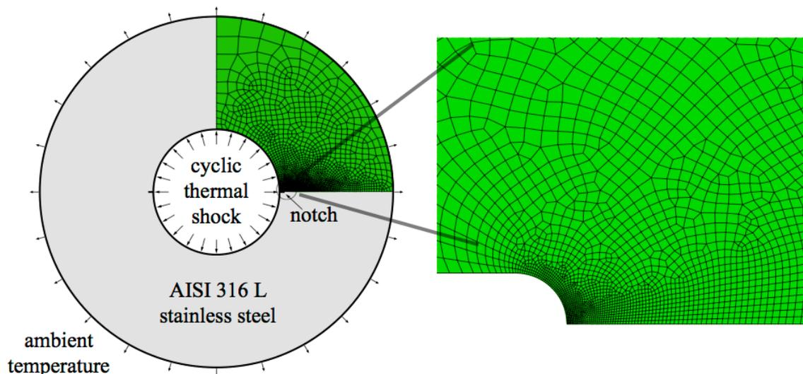
Figure 2. The geometry and the finite element mesh of the notched ring specimen submitted to cyclic thermal shocks.
