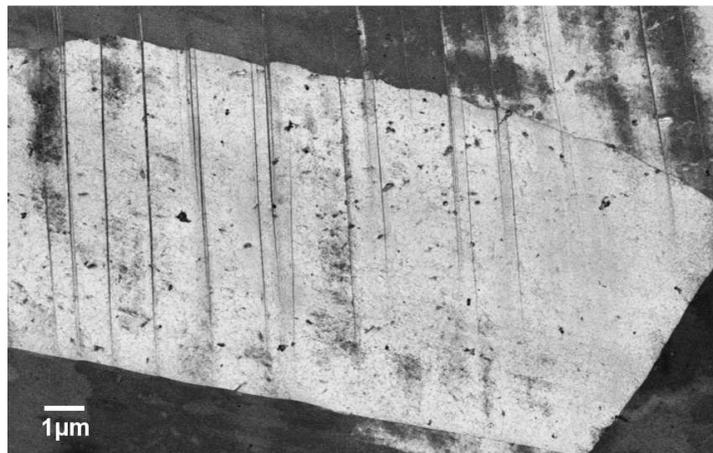
Figure 8: Inverted ECCI micrograph for a specimen with tension-torsion deformation on the circle path and 1% equivalent strain at  $N_f=45$  cycles showing area with additional strain localization (micro twins).
